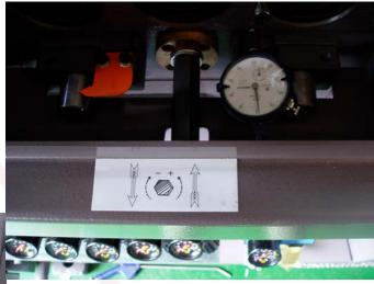
3. Adjustment for the feeding locations: The feeding locations shall only be adjusted if a loud striking sound is produced during working or vibration is produced when the wood is hit by the saw blade moving upward – otherwise, the adjustment is not required. (Most wood material can be cut via the factory setting)
