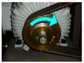
5. Make sure the motor rotates to the right direction.
