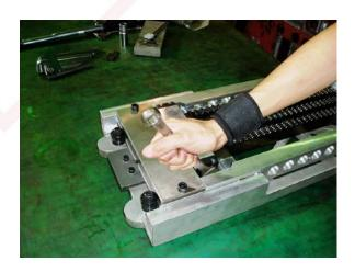
(2. Loosen the blades by pulling upward the handle in  $90^{\circ}$ )
