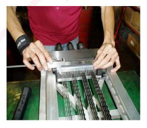
(14. Check the parallelism between the saw blades)
