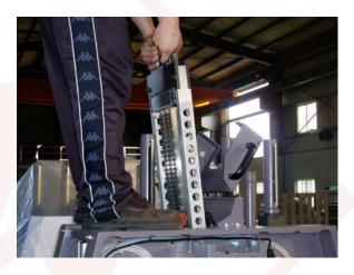
2.1 install the immovable axle that add spacer to underside hole when using 200mm frame (saw blade is 500mm in length)
