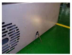
2. Install the frame and tighten the frame to 60Nm with a torque wrench. Withdraw the pin.
