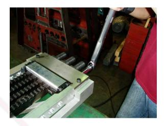
Loosen the push bolts, and knock the push bolts loose with a hammer.
