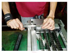
(12. Check the parallelism between the saw blades and the frame)
