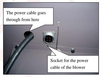
(The power cable inlet and the socket for the power cable of the blower)
