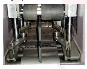
4. Please use the right side holder while the front middle feeding grate plate is to be mounted by the side. Long side holder wheels can be used if required.
