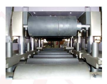
Replace method: Loosen the retaining screws M6 under the fixing plate of the pressing wheels, loosen the retaining screws for the pressing wheel slides, and take off the pressing wheels. Take off the snap rings with a snap ring plier and replace the snap rings.
