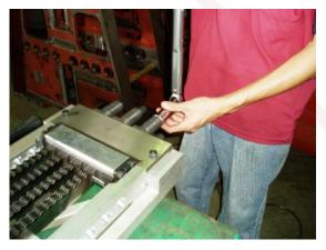
(11. Adjust the torque wrench to 120Nm)
