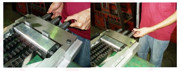
(4. Insert into the clearance with four 5mm shims, and then properly screw these three nuts with hands so that the clearance becomes 10mm. Withdraw the shims)
