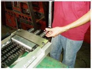
(Adjust the torque wrench to 120Nm)
