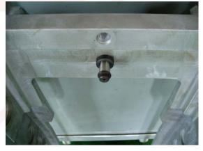
2.2 install the immovable axle to top hole when using 250mm frame (saw blade is 550mm in length)
