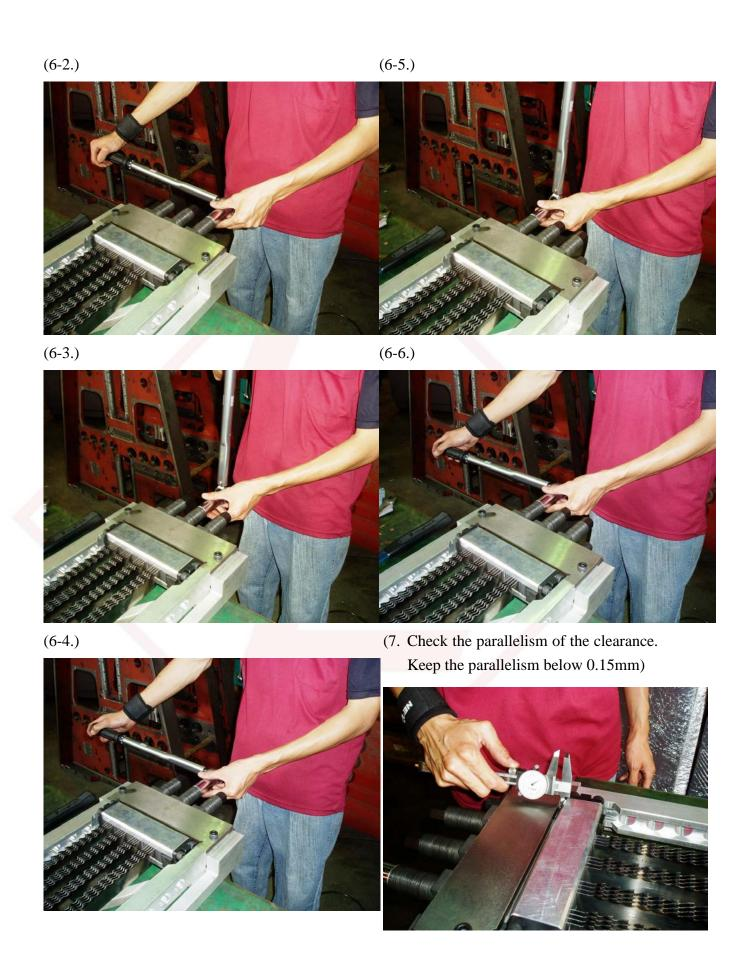
(8. The parallelism error of the clearance can be corrected with the three draw-in bolts)
