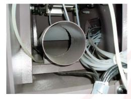
(The front dust-suction port is hidden in the inner side at the lower part)
