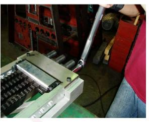
(5. Screw the push bolts to 35Nm – the saw blades are not fully clamped at this time)
