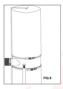
PLACE THE COLLECTOR AND FILTER BAGS ONTO THE COLLECTOR AND SECURE WITH THE BELTS AS SHOWN IN FIG.9.
