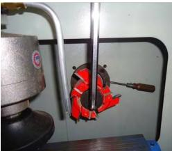
After the milling cutter axis move to suitable position, the tool insert to the groove from the end cover hole of the main shaft (e.g. screwdriver), to prevent the rotation of the spindle. Please see the right picture.
