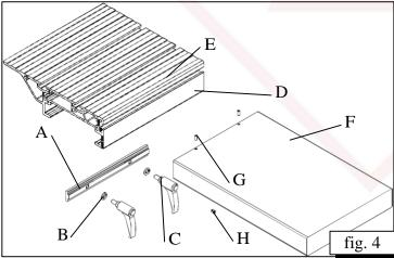
Assembly guiding wedge A (fig. 4) (together with washers B and handles C) in "T- channel" D on the moving table E.
