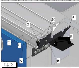
Assembly of the handle for the moving of the movable table
