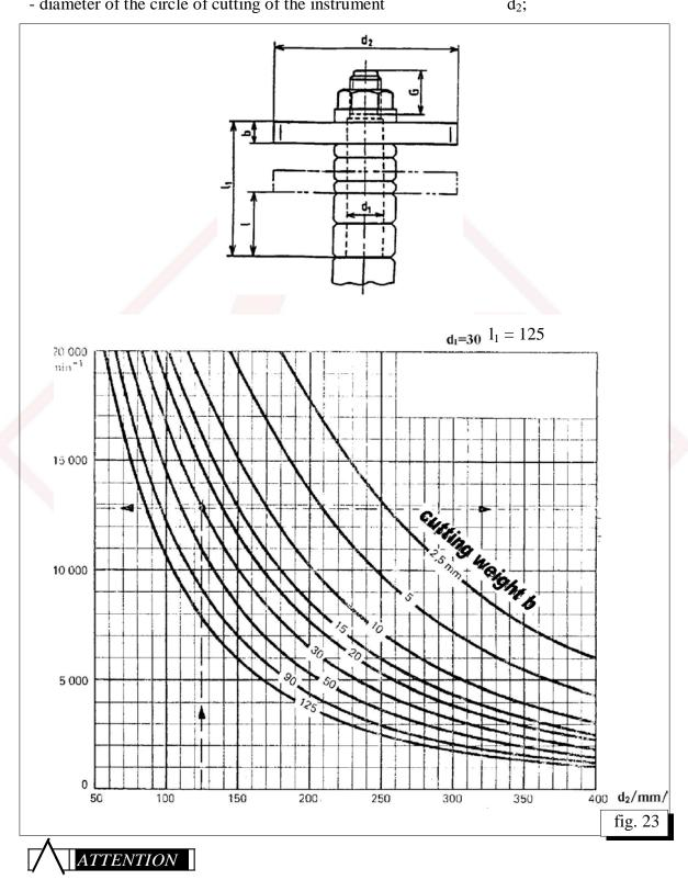
The operating rotations of the spindle must not exceed the maximum permissible ones as recommended be the producer.
