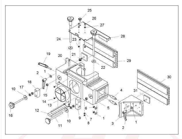
PF180-00.00.00-01 PROTECTION DEVICE Ø180MM WITH INTEGRAL RULERS (OPTION)
