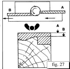
If the profiling is not done along the whole length of the piece, both supporting rulers will level. (fig. 28)
